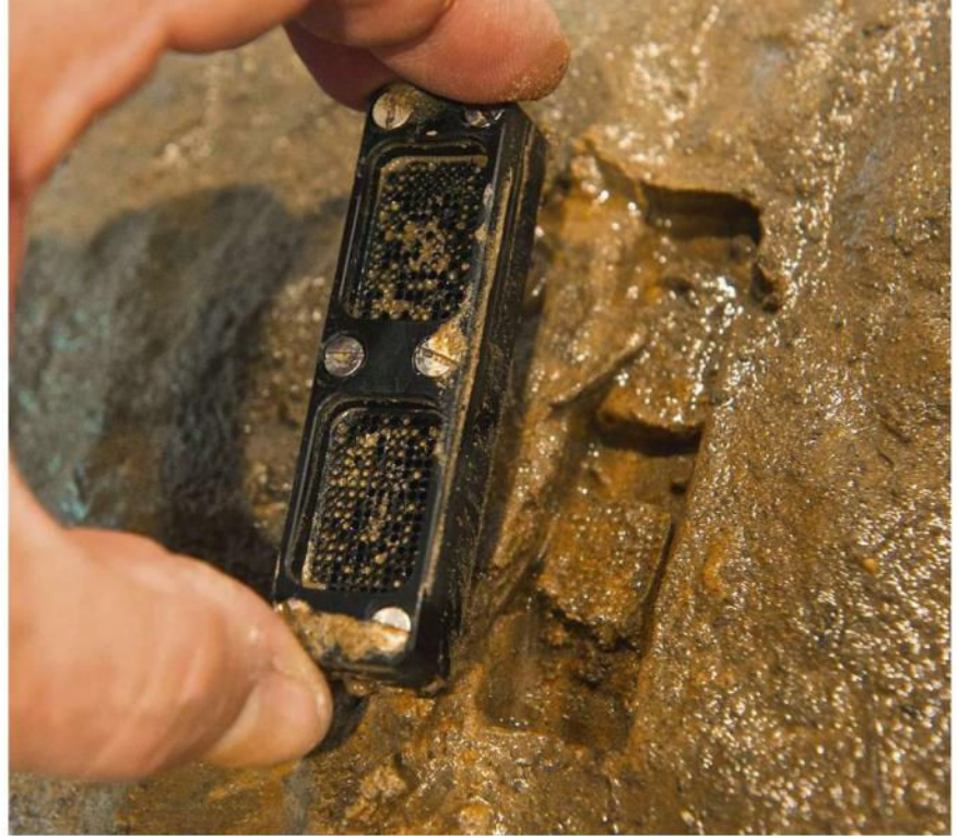
ISOLATION CHIP This small, plastic block contains hundreds of tiny wells in which bacteria multiply to create hundreds of colonies that scientists can study
