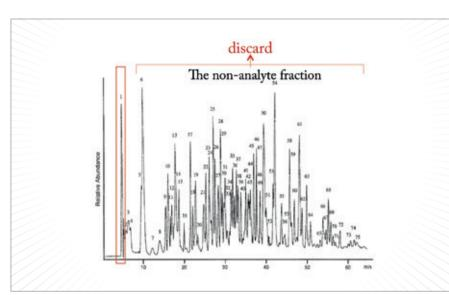
Figure 2. An MASC solution to the problem illustrated in Figure 1. The red box is where affinity selected analytes would coelute. All other substances would be discarded before entering the mass spectrometer. Adapted from Reference 3 (peaks highlighted in Figure 1 have not actually been removed from Figure 2).
