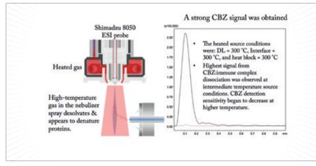
Figure 5. The inlet system used in ESI-MS analysis of carbamazepine.
