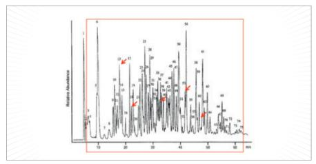
Figure 1. An illustration of problems encountered in LC-MS analysis of small numbers of analytes in complex biological samples. Red arrows show targeted analyte elution positions while the red box contains analytes that enter the mass spectrometer. Adapted from Reference 3 (highlighting added).
