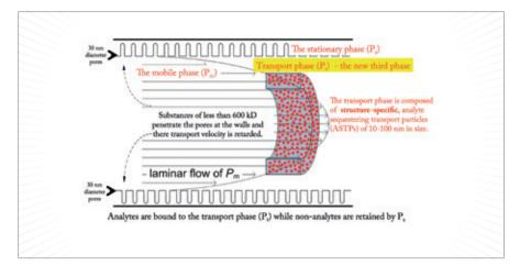
Figure 3. An illustration of the mobile affinity sorbent chromatography (MASC) model, demonstrating the three phases involved in separation processes. The function of the transport phase (Pt) is to sequester and accelerate the elution of analytes while that of the stationary phase (Ps) is to bind and retard elution of non-analytes. The mobile phase regulates partitioning between these two phases. This rapidly separates analytes from non-analytes.
