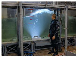
**FIGURE 1. THE BREAKING LABORATORY WAVE** seen here is moving from right to left and is lit from beneath. We analyzed turbulent, air-entraining flow in white, foamy wave regions like that shown just below the water surface. Electrical engineer James Uyloan helps show the scale of the experiment.
