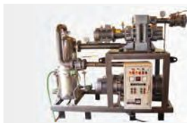
Roots pumping system
