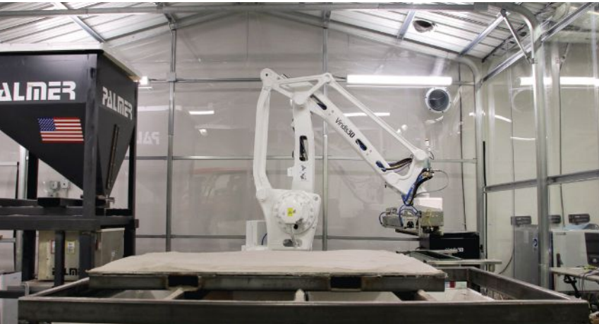
Figure 3: Robotic additive manufacturing system uses a proprietary 3-D printing process to produce sand molds and cores for the metal casting industry. Courtesy: Viridis3D/RIA
