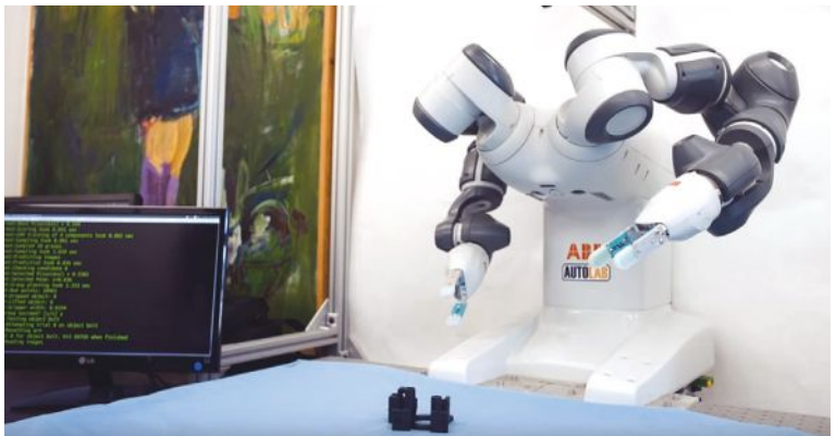
Figure 3: A robot manipulates objects it has never encountered before after researchers teach a neural network how to recognize objects from millions of 3-D models and images. Courtesy: University of California, Berkeley/RIA
