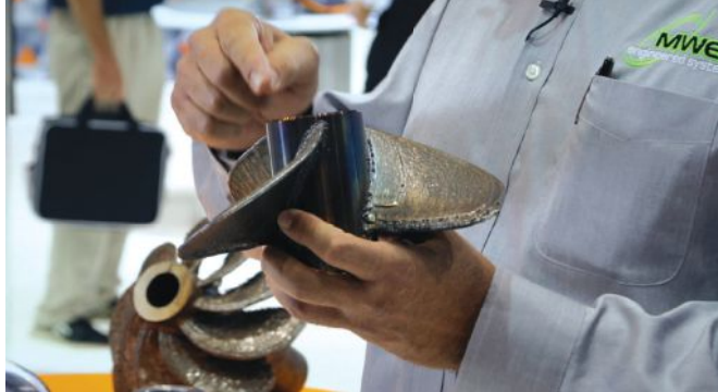
Figure 2: Propeller blades built with a robotic laser additive manufacturing process shown near net shape before finishing. Courtesy: Midwest Engineered Systems Inc./RIA
