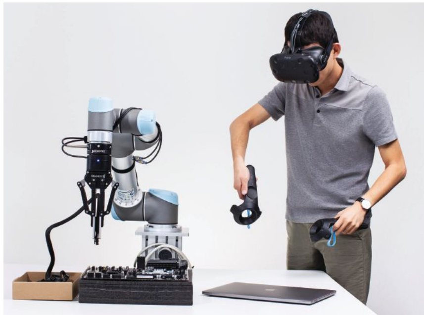
Figure 5: Operator wearing a VR headset and holding motion-tracking devices teleoperates a robot, showing it how to grasp and manipulate objects so it can learn how to perform new skills on its own using reinforcement learning. Courtesy: Embodied Intelligence/RIA
