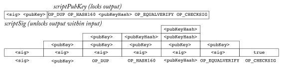
**Figure 4.2:** Example execution of a Pay-to-Public-Key-Hash (P2PKH) Bitcoin script in one transaction input.
