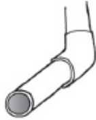
45° elbow friction loss equal to 2.0' straight pipe
