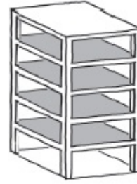
Floor diaphragm extra stiff construction resists horizontal forces across the plane of the floor
