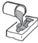
Casting/molding A molten or liquid material is placed in a mold to solidify
