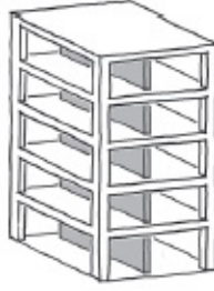
Shear wall extra stiff construction resists lateral forces in the direction of its surface
