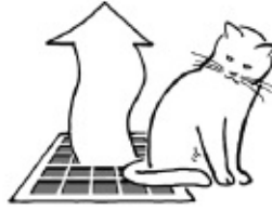
Convection heat transfer through move- ment of a fluid (air or liquid)
