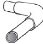
90° elbow friction loss equal to 4.0' straight pipe
